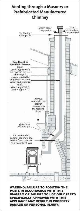
Figure 6. GF 300 BV venting through a masonry chimney.
